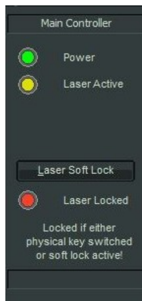
Fig. 16: Laser hard locked (key switch or interlock)
