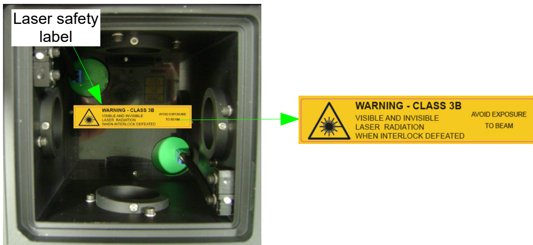
Fig. 1.2: Safety label of the Multi Channel Detection Unit after removing the filter holder. Once the filter holder is removed, laser radiation of laser class 3B can occur inside the housing when interlock defeated.
