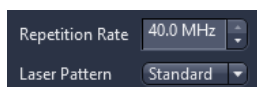
Fig. 3.9: Repetition rate can be adjusted in the “Laser Settings” of the Zeiss PicoQuant application
