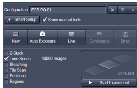
Fig. 2.17: Start of the point measurement in the LSM software. The measurement is started by clicking on "Start Experiment". Note that the button is only active, if the “Time Lapse” Box is checked (left).
