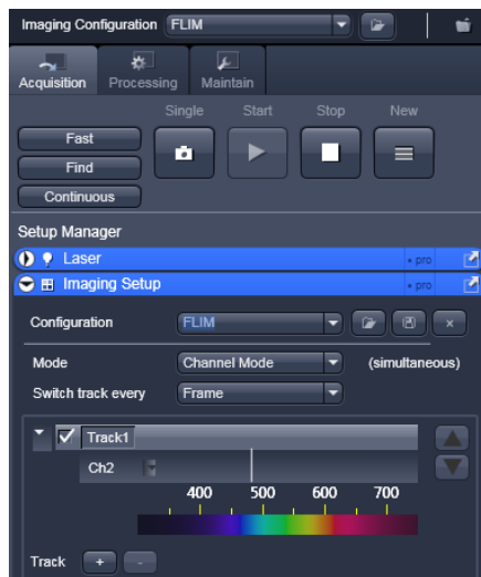
Fig. 2.11: Storing and applying stored configurations is possible via the “Imaging setup” tab. Clicking the “open” icon in the “Configuration” line opens a stored configuration. Entering a new configuration name and clicking on the “save” icon stores the actual configuration.
