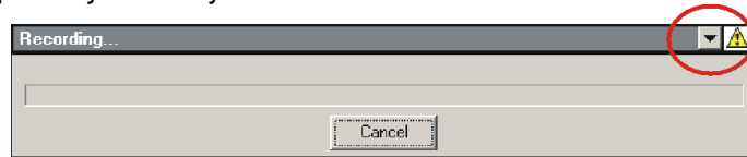
Fig. 3.7: SymPhoTime Pop-up-window being displayed during LSM data recording. To see the image during acquisition, press the button .
