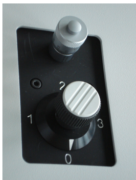
Fig. 2.18: Laser attenuation at the LCU: rough adjustment at the intensity can be performed with the filter wheel. the position correspond to the following attenuations: 0=no attenuation (max. power), 1 = 10x attenuation, 2 = 100x attenuation, 3 = 1000x attenuation. The upper knob controls the scaffold for intensity fine tuning. Turning the knob clockwise moves the scaffold into the laser beam and thereby attenuates the excitation intensity.
