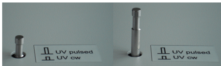
Fig. 3.1: LCU settings for standard confocal operation using the cw lasers of the LSM (left) and pulsed excitation for FLIM (right).
