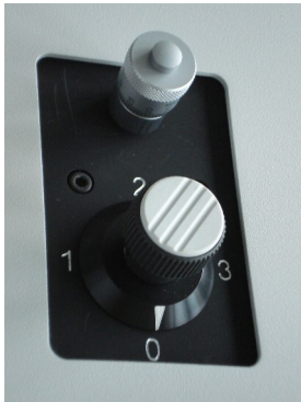
Fig. 2.11: Laser attenuation at the LCU: rough adjustment at the intensity can be performed with the filter wheel. the position correspond to the following attenuations: 0=no attenuation (max. power), 1 = 10x attenuation, 2 = 100x attenuation, 3 = 1000x attenuation. The upper knob controls the scaffold for intensity fine tuning. Turning the knob clockwise moves the scaffold into the laser beam and thereby attenuates the excitation intensity.
