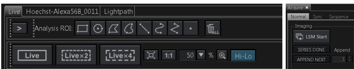
Fig. 2.13: Starting a pre-selected point measurement in the FV3000 software by clicking “Live” for measurements which should be stopped manually.
