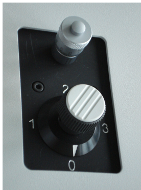
Fig. 2.20: Laser attenuation at the LCU: rough adjustment at the intensity can be performed with the filter wheel. the position correspond to the following attenuations: 0=no attenuation (max. power), 1 = 10x attenuation, 2 = 100x attenuation, 3 = 1000x attenuation. The upper knob controls the scaffold for intensity fine tuning. Turning the knob clockwise moves the scaffold into the laser beam and thereby attenuates the excitation intensity.
