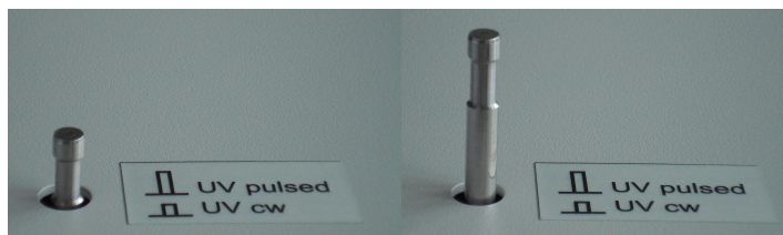
Fig. 2.1: LCU settings for standard confocal operation using the cw lasers of the LSM (left) and pulsed excitation for FLIM (right).
