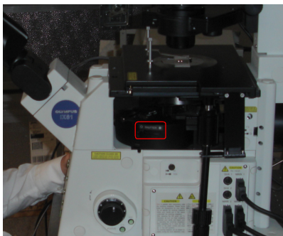
Fig. 2.16: mechanical shutter at the Olympus IX81 microscope
