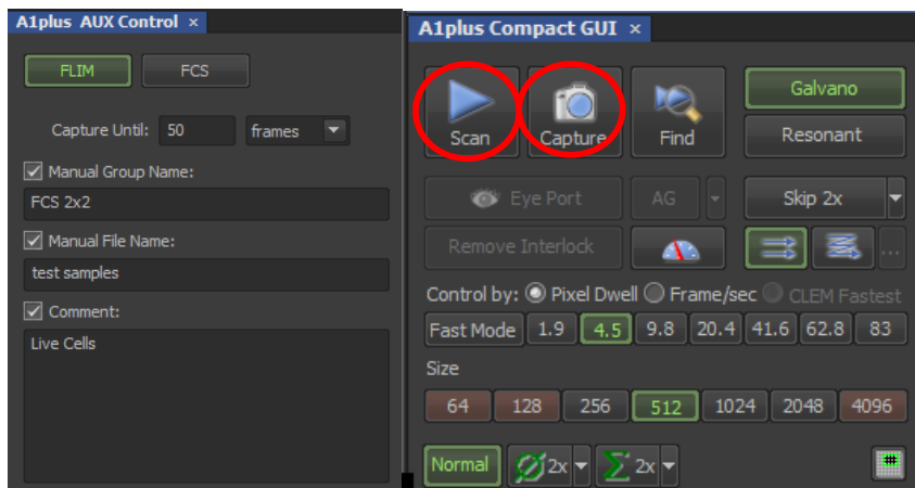
Fig. 2.25: Selection of a FLIM measurement up to 50 frames, and controls to start the measurement. “Scan” makes a test measurement, which is not saved, and “Capture” makes a final measurement which is saved.
