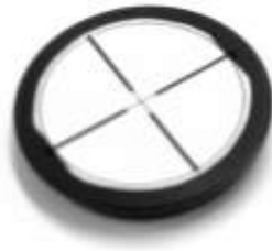
Fig. 5.6: Alignment tool for detector unit alignment
