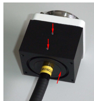
Fig. 5.3: Complete NDD adapter. The inner part of the adapter should flush with the outer part (red arrow). The two screws fix the inner part of the adapter.
