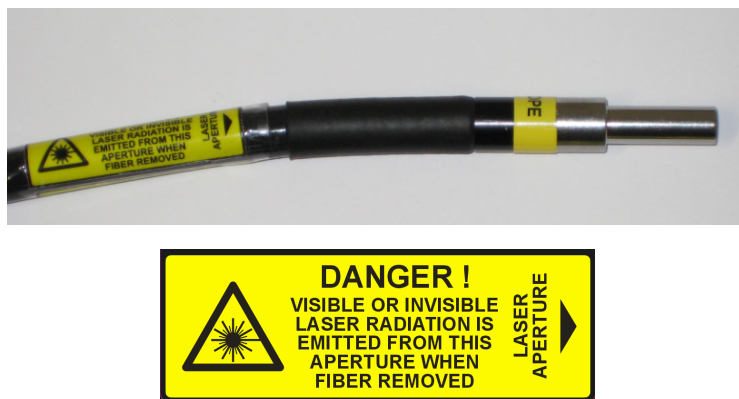
Fig. 1.3: Safety labels on light guide connecting the NDD adapter with the detection unit: LASER APERTURE and Laser safety label.
