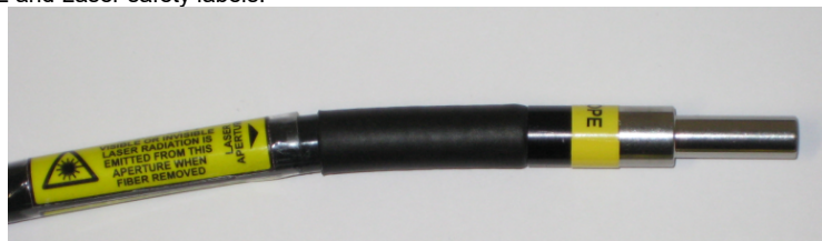
Fig. 1.1: Safety labels: LASER APERTURE and Laser safety labels.
