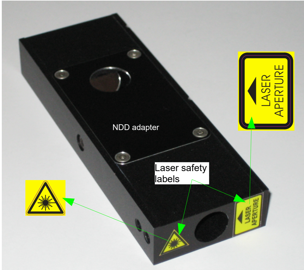
Fig. 1.1: Safety labels: LASER APERTURE and Laser safety labels.
