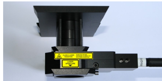
Fig. 5.3: NDD adapter with two extension tubes, each adding 10 mm. The additional height is now 67 mm.
