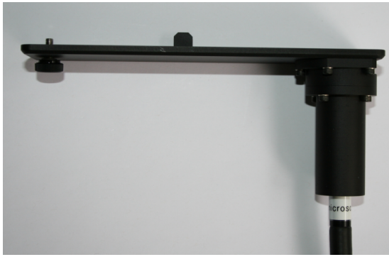
Fig. 5.3: NDD adapter cover. Replace the standard cover of the NDD detection unit with this one for FLIM measurements.
