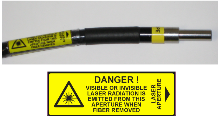
Fig. 1.2: Safety labels on light guide connecting the NDD adapter with the detection unit: LASER APERTURE and Laser safety label.
