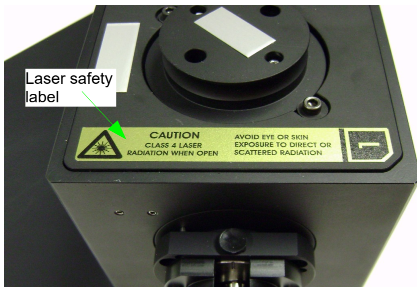
Fig. 1.1: Safety label on top of the Multi Channel Detection Unit.
