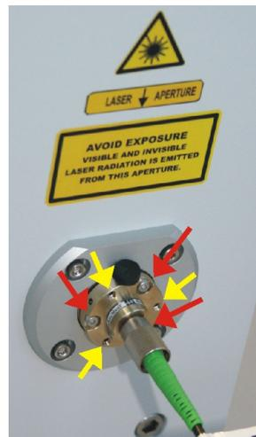
**Fig. 5.9:** Fiber Outcoupling Unit at the dual detector unit. the adjustment screws are marked in red, the counter screws are marked in yellow.
