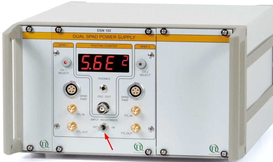
Fig. 4.3: DSN 102 dual SPAD power supply (optional)
