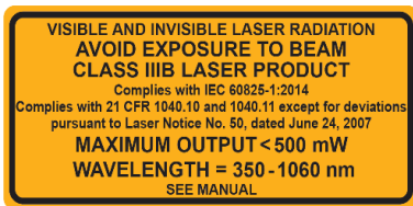
Fig. 1.5 Class IIIB Laser Power and Wavelength Specifications Label on the side of the LCU (B)
