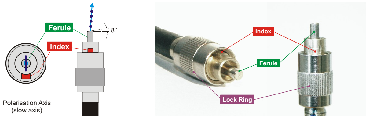
Fig. 2.13: Standard FC-APC connector with 8° angled polish which is rotated by 90° to the connector index. With the standard PM-SM-fiber of the LCU the used polarization axis of the fiber is orientated as demonstrated on the left hand side. The polarization plane of the laser beams are parallel aligned to this axis.
