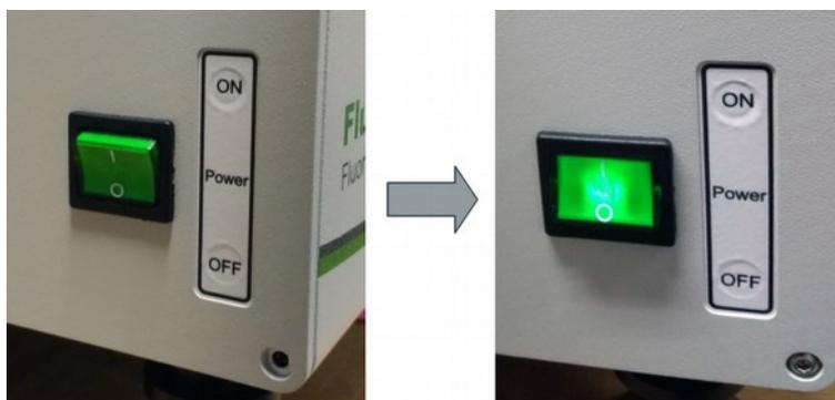
Fig. 26: Turning the FluoTime 250 on.
