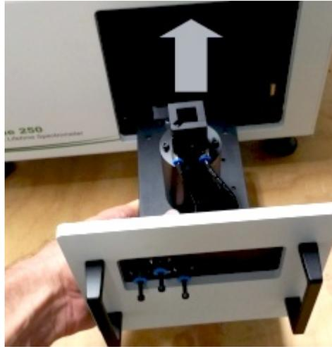
Fig. 24: Sliding a sample mounting unit into the FluoTime 250
