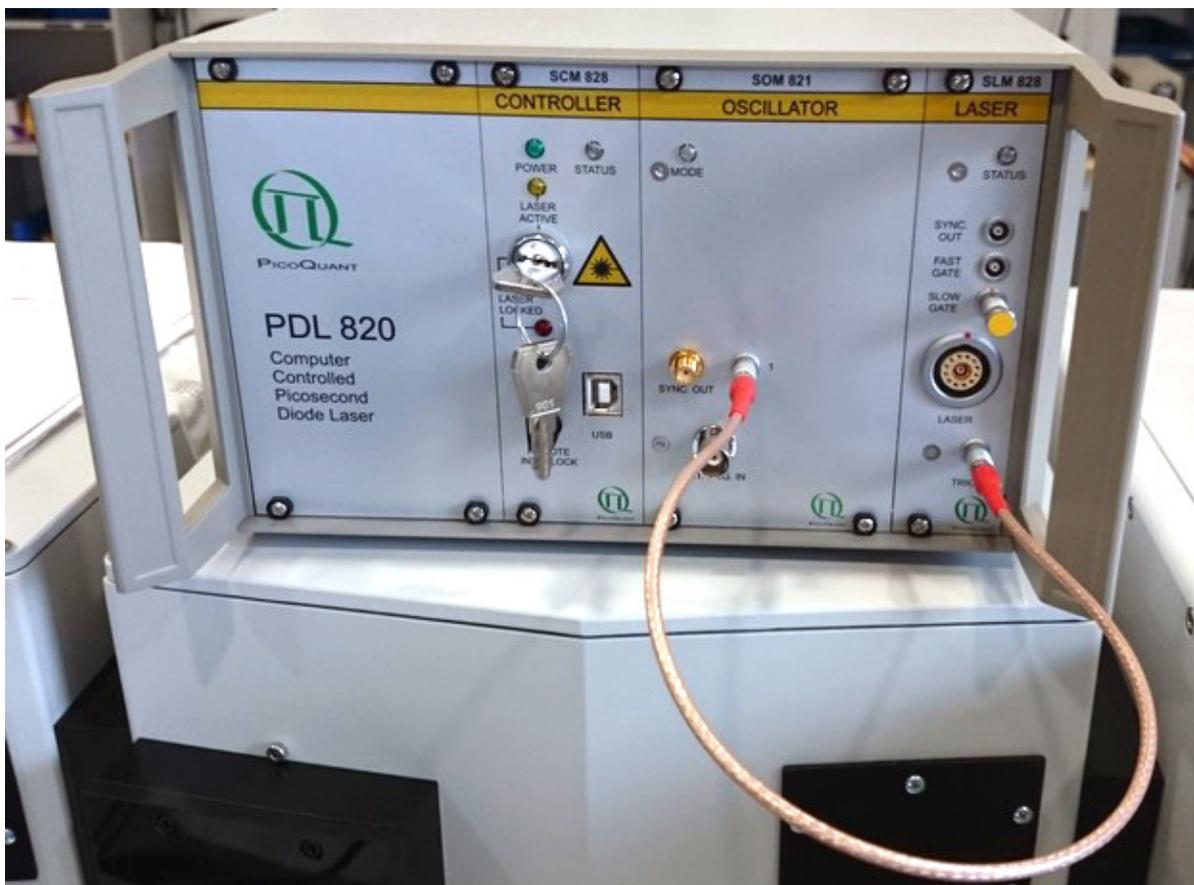
Fig. 9: Trigger cable at the PDL 820.
