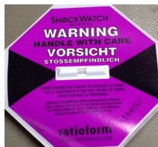
Fig. 4: Shockwatch sensor.
