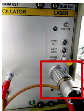
Fig. 23: Connection of the light source to the PDL 820 laser driver.
