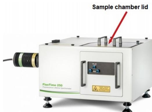
Fig. 25: Sample chamber lid of the FluoTime 250
