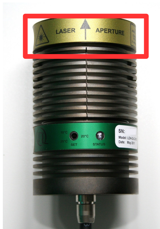
Fig. 1.1: Example of laser warning, certification, and classification label on laser heads of the LDH Series. Top: labels for cylindrical laser heads; bottom: location of such a label on a laser head from PicoQuant's LDH Series.
