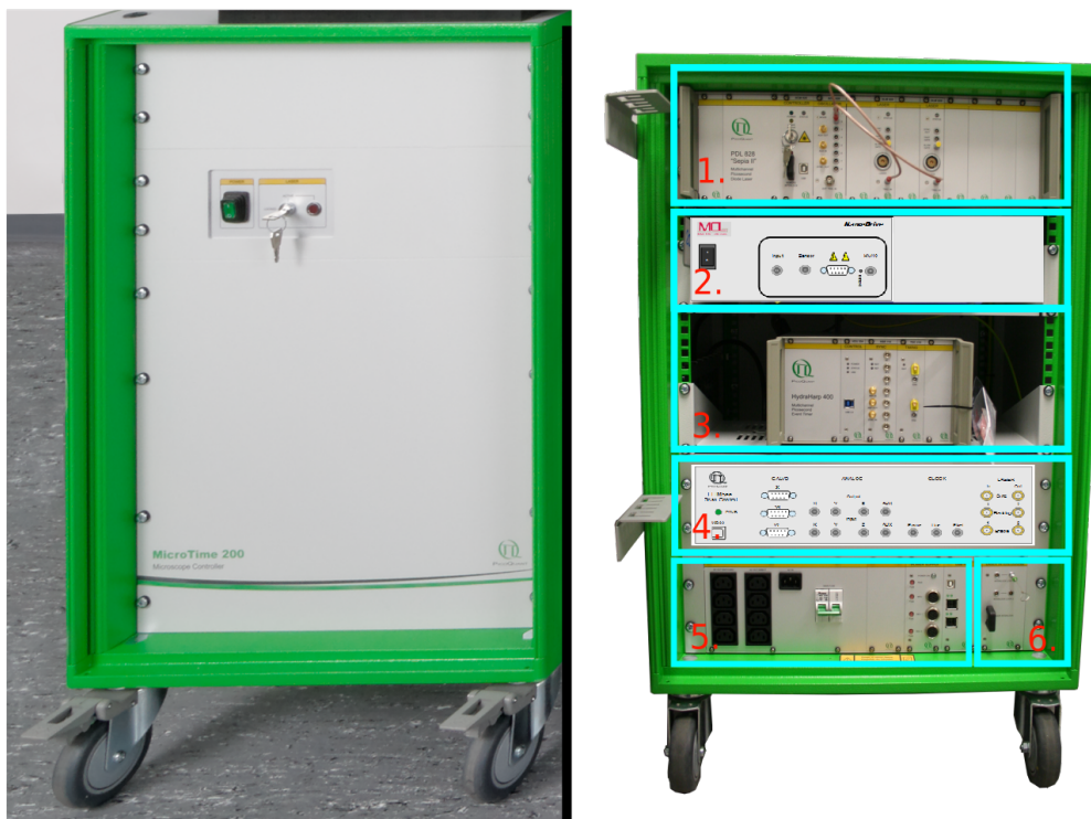
Fig. 2.5: Microscope controller 19" rack front side (left) and back side (right) showing the control electronics for the MicroTime 200 and FLIMbee Galvo Scanner
